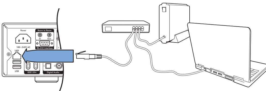
High Definition media files are high bandwidth when streamed across the network and a 100Mbit/s (100BASE-T) network is therefore recommended.
