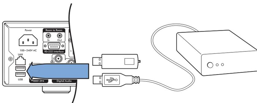
*Crystalio II Media Player* supports the use of USB 1.0 and USB 2.0 Mass Storage Devices. This term can refer to thumbdisks, external HDDs with a USB interface and other devices that are seen by *Crystalio II* as file storage.
